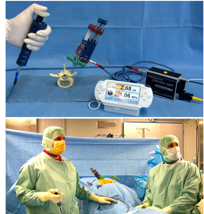
Vertebral cement injector Loeffel-M, thesis, Univ. Bern (CH), 2007.
