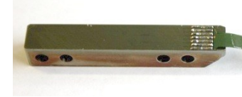
Thin-film force sensor for spinal distractor Ambrosetti-Giudici-S, thesis, Univ. Bern (CH), 2009.
