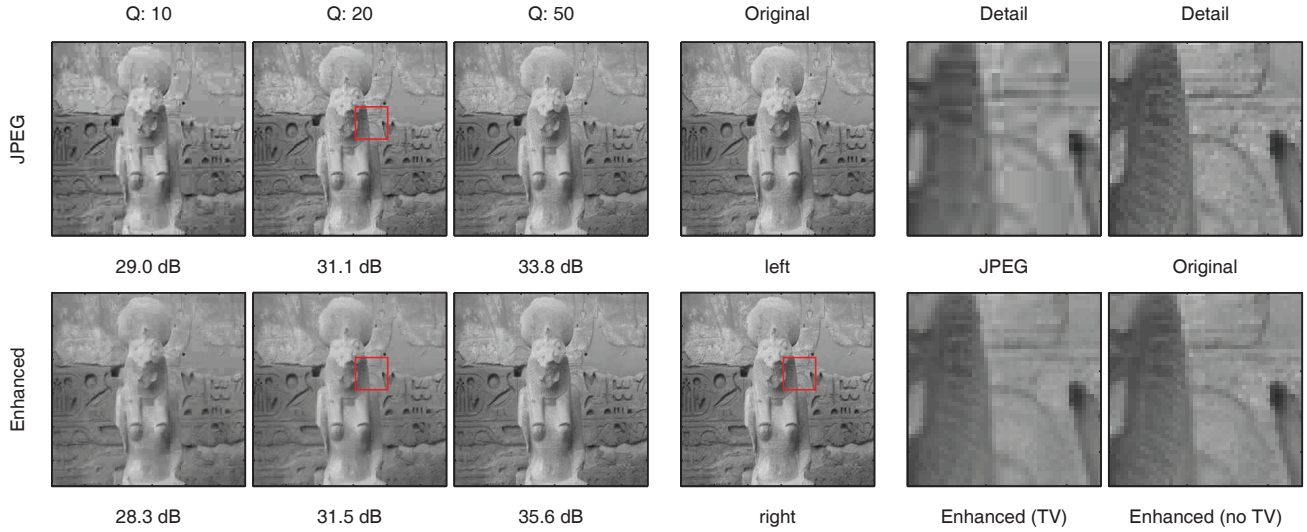
Fig. 2. This experiment on a 288 \times 288 pixel image of Sekhmet taken with a commercial stereo camera illustrates our method. Results for three different JPEG quality settings with and without enhancement are followed by the original left and right view and enlarged details from the second image pair. We can improve the visual quality even if PSNR results drop and find less blocking artifacts if the total variation of the disparity field is minimized. Compare these results with Fig. 3(a).
