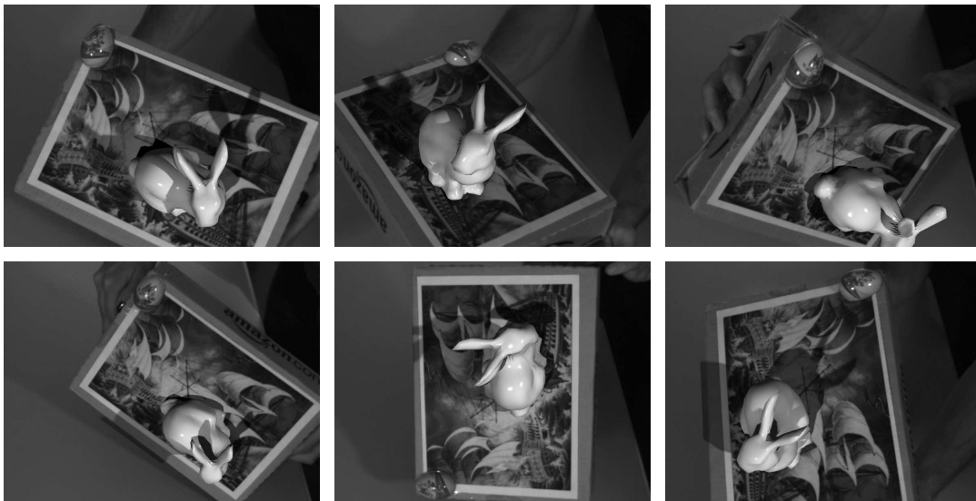
Fig. 14. The synthetic rabbit has been added to the other images of the video without re-computing the light sources. The result remains realistic and we provide the corresponding video as supplementary material.
