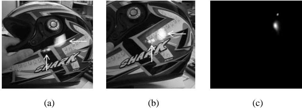
Fig. 8. Extended sources detection. (a,b) Two input images of a helmet lit by two extended light sources, one being more so than the other. The arrows point toward the main specularities. (c) The accumulator obtained after applying the method of Section 3.1. The widest peak corresponds to the most extended source. In our current scheme, the brightest pixel of this peak will represent the source.
