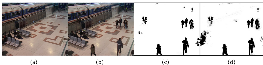
Fig. 6. PETS 2006 Dataset. (a) Initial frame of the video, used as background model. (b) Frame number 2800. (c) The background subtraction of [1]: The abandoned bag in the middle of the scene has mistakenly been integrated into the background. (d) Our method correctly segments the bag, the person who left after sitting on the bottom left corner, and the chair that has been removed on the right.
