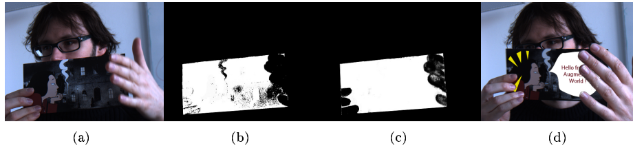
Fig. 7. Occlusion segmentation on a moving object. (a) Input frame in which the card is tracked. (b) Traditional background subtraction provide unsatisfying results because of the shadow cast by the hand, and because it learned the fingers hiding the bottom left corner as part of the background. (c): Our method is far more robust and produces a better segmentation. (d) We use its output as an alpha channel to convincingly draw the virtual text and account for the occluding hand.
