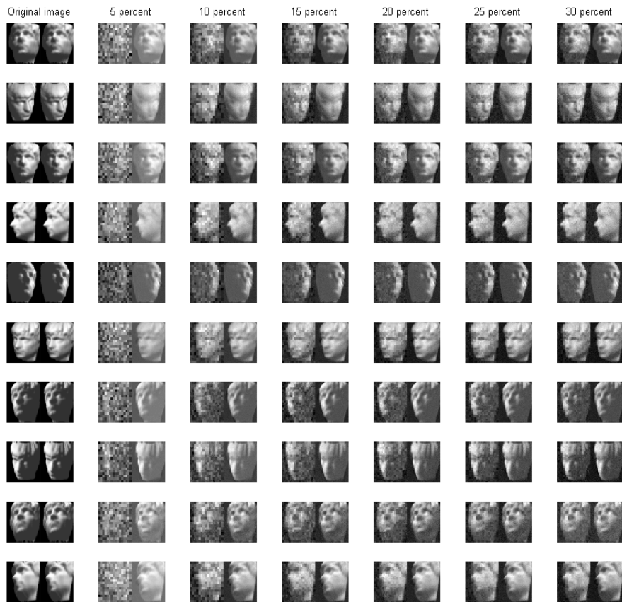
Fig. 2. Sparse signal recovery performed on a mixture of factor analyzers (MFA) model, inferred based on training data using Dirichlet process (DP) and beta process (BP). The left-most images are the original data, and the other columns represent CS recovery, based on random compressive measurements. Results show performance when the number of CS measurements are 5%, ..., 30% of the total number of pixels in the image. In columns two through seven, the left figure employs the CS-recovery algorithm in [29], which does not exploit the MFA, and the right image is based on the learned MFA. [Results courtesy of M. Chen.]
