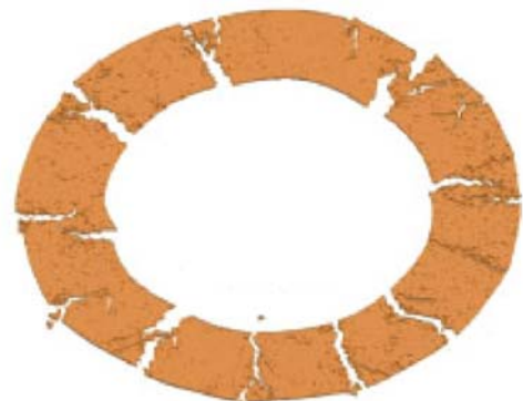
Fig: Fragmentation of a ring under high loading
