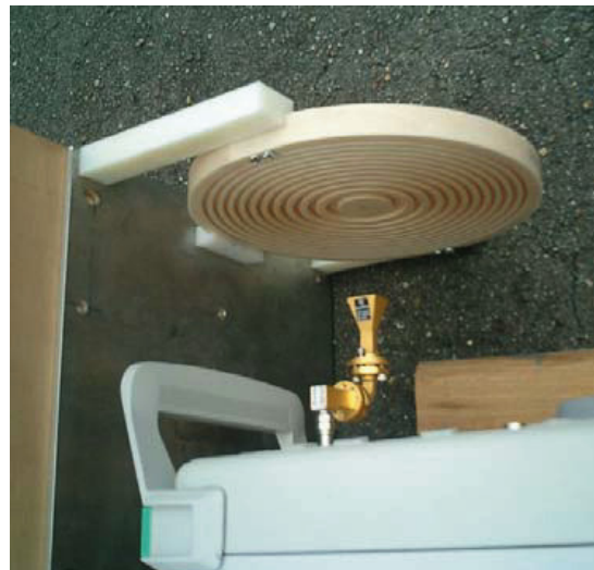
Figure 16. Top view of the Fresnel lens transmitting antenna illuminated by the horn.
