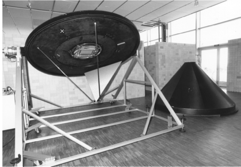
Figure 2: Bi-directional photogoniometer developed at LESO-PB/EPFL. The CCD camera (absent on the picture) is fixed on the rotating ring at the cross mark.
