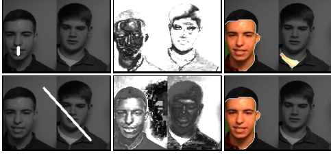
Fig. 2. Segmentation results [right] when using the regional term in previous methods [top] and our regional term [bottom] given the manually-added seeds [left] and corresponding probability maps [center] for foreground [top] and background [bottom]. No audio-visual term is used in this comparison ( \lambda_C = 0 ). The foreground is shown in brighter grayscale. White regions represent the seeds [left] and a low probability [center].
