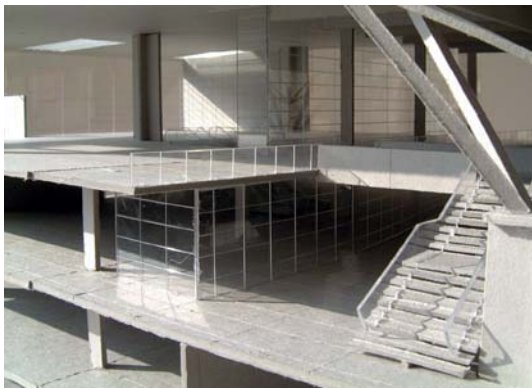
Fig. 2: Study of sunlight penetration inside a scale model
