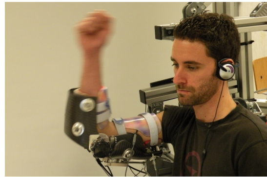
Fig. 5. Front view of a participant wearing the NEUROExos.
