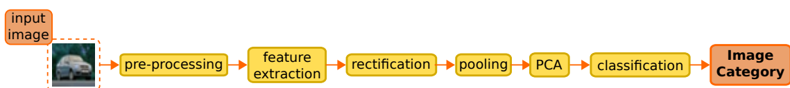
Figure 1.1: Our pipeline, similar to many recent approaches. We tried different options for each of the different steps, in order to evaluate the importance of sparsity constraints in the Feature Extraction step, and the impact of the overall architecture on the recognition rate.
