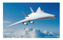
(+) reduced fuel consumption, because of reduced drag. Some open issues for cargo (shape), frontal surface still important.
