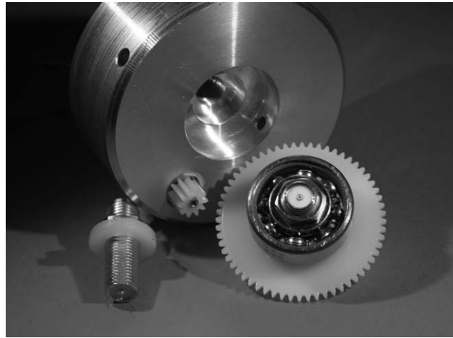
Figure 2 First prototype of the rotary joint (bottom left: fixed SMA section; bottom right: rotating SMA section hold inside the ball bearing; and behind: aluminum cylindrical structure with electromotor and pinion)
