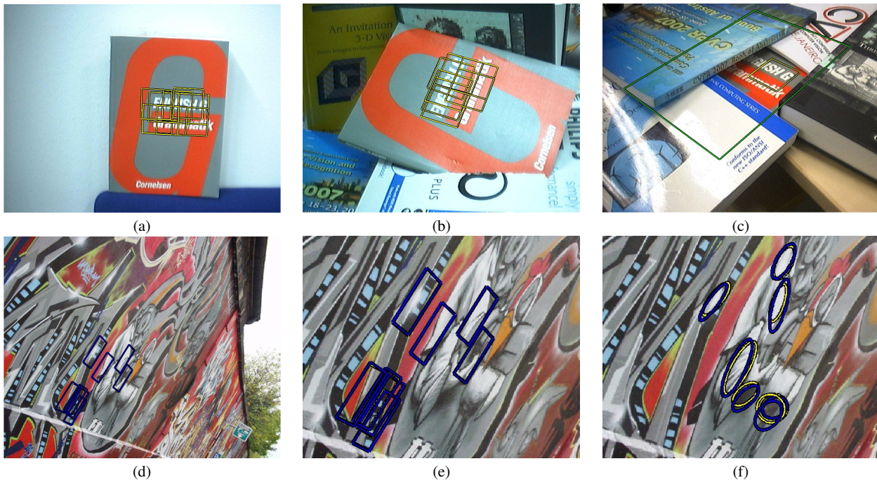
Fig. 1 The advantages of learning for patch recognition and pose estimation. (a) Given a training images or a video sequence, our method learns to recognize patches and in the same time to estimate their transformation. (b) The results are very accurate and mostly exempt of outliers. Note we get the full perspective pose, and not only an affine transformation. (c) Hence a single patch is often sufficient to detect objects and estimate their pose very accurately. (d) To illustrate the accuracy, we use the ‘Graffiti 1’ image and the ICCV booklet cover respectively to train our method and detect patches in the ‘Graffiti 6’ image and in the real scene respectively. We then superimpose the retrieved transformations with the original patches warped by the ground truth homography. (e) Even after zooming, the errors are still barely visible. (f) By contrast, the standard methods retrieve comparatively inaccurate transformations, which are limited to the affine transformation group.
