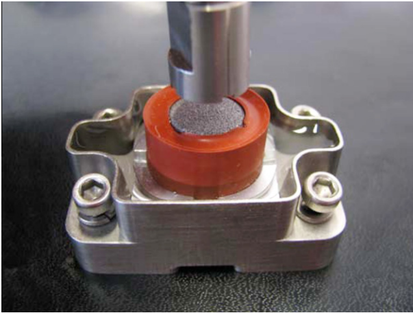
Fig. 1. Experimental set-up for confined compression showing the centering plate in the immersion tank, the silicon membrane and the porous plates enclosing the hydrogel sample allowing fluid flow.
