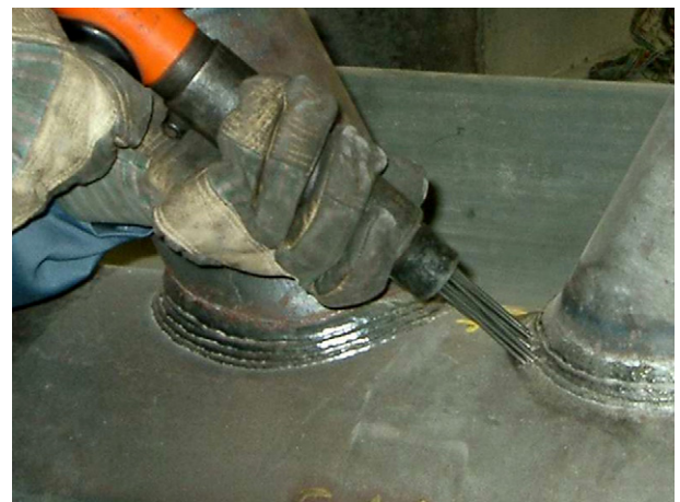
Fig. 3. Needle peening of test specimens [1].
