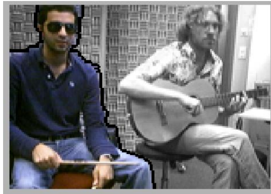
Figure 2.2: Segmentation of one frame: foreground is depicted in the RGB color space; background is shown in gray scale; a black contour is drawn to better observe the difference between them.
