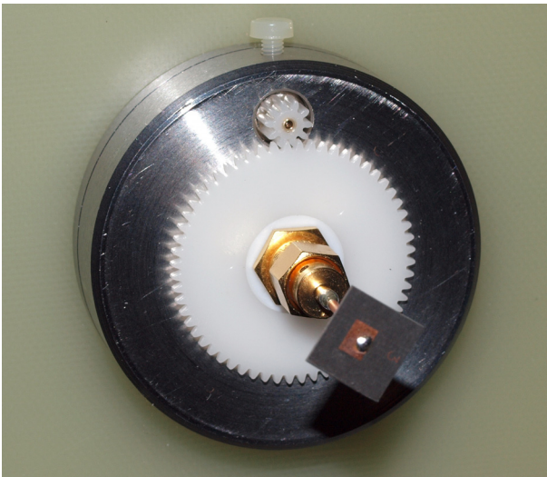
Figure 6: the second rotary joint with a 30 GHz patch (outer diameter of the device: 50 mm)
