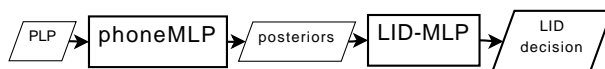
Figure 3: The hierarchical approach. The “phoneMLP” is shown in Fig. 1 and the “LID-MLP” is sketched in Fig. 4.
