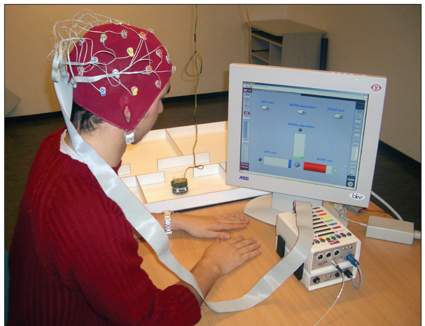
Fig. 2. Noninvasive BMI based on the analysis of EEG signals, i.e., the brain electrical activity recorded from electrodes placed on the scalp (colored spots in the red cap worn by the person). The user is mentally driving a mobile robot between rooms in a house-like environment, making it turn or move forward. Alternatively, he can control some software processes running in the computer by triggering the same EEG patterns as for the interaction with the robot.
