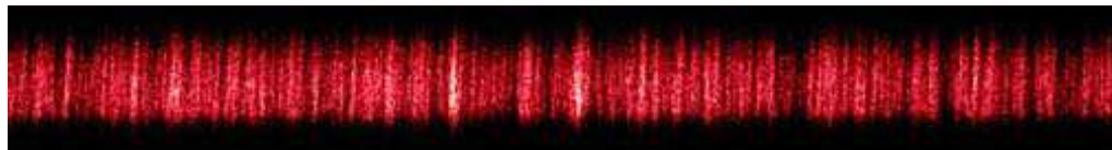
Fig. 4. Photo of a section of the intensity distribution for a 1D diffuser showing the non periodic intensity variations.
