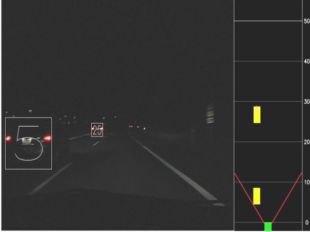
Figure 1. Sample output of our Real-Time Tracking System. On the left part tracked vehicles are marked and their distance in meters to the camera is overlaid on them. On the right part a radar-like view of the scene is drawn: A green rectangle represents the car on which the camera is mounted and yellow rectangles represent other vehicles. The purple segment on them indicates their relative velocity with respect to the camera.
