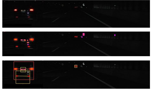
Figure 2. Detection Results. Top Row: Input frame. Center Row: Taillight Detection. Bottom Row: Vehicle Detection.
