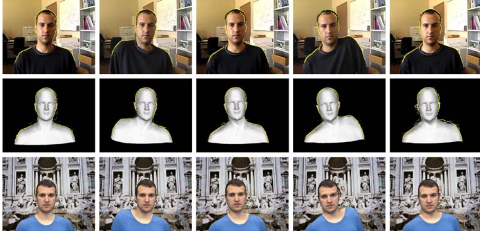
Figure 15. Tracking of the moving head and shoulders in a 125-frame sequence. Top row: Images from the original video sequence with detected silhouette edges overlaid. Second row: Recovered model's shape shown as the shaded model in the same position as the original images above. Bottom row: Recovered model placed in front of a different background.
