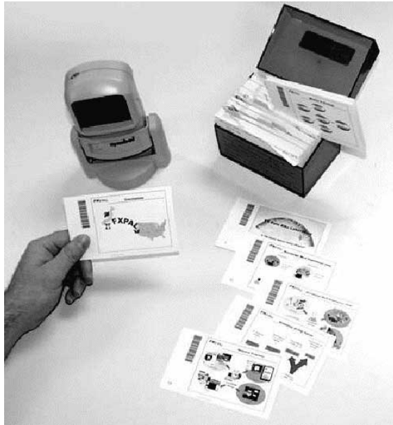
Figure 3.6: Elements of the Palette system [Nelson et al., 1999], which allows presenters to control slideshows with printed cards. The content of the slide is printed on the corresponding card. To display a slide, users simply show its card to a card reader (top left device).
