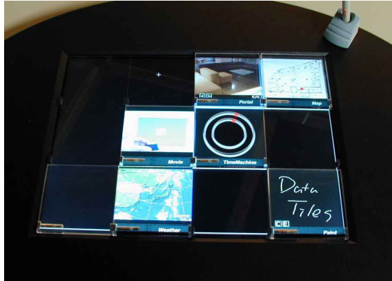
Figure 2.11: Several DataTiles [Rekimoto et al., 2001] arranged on a tray. The two illuminated circles are engraved in the tile to facilitate pen-based interactions.
