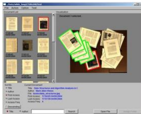
Figure 3.3: Snapshot of the desktop application of the video-based document tracking proposed by [Kim et al., 2004]. It allows users to browse through the stacks of documents placed on an office desk.
