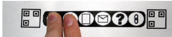
Figure 3.4: The command bar printed on each document in the system proposed by Smith et al. [Smith et al., 2006]. It allows users to issue commands by hiding the corresponding icon.
