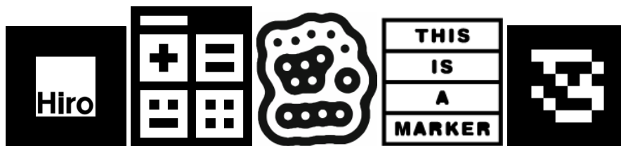
Figure 6.10: Examples of fiducial markers. From left to right: Artoolkit, d-touch (original), reacTIVision, d-touch [Costanza and Huang, 2009] and Artag.
