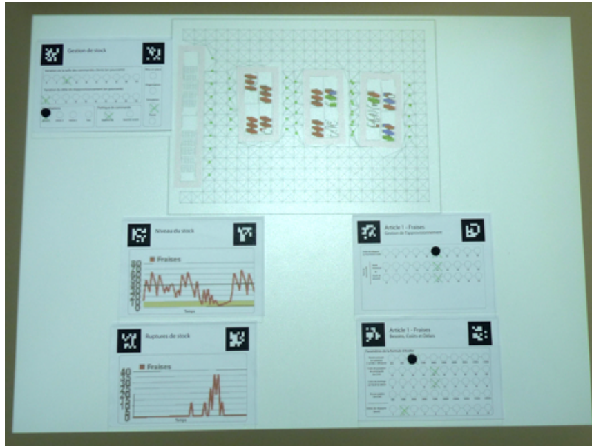
Figure 6.16: Module 3: The simulation adapted for storage management activities. The small-scale model is not used anymore and the warehouse is displayed four times smaller than usual to leave space for TinkerSheets arranged around it. These TinkerSheets allow apprentices to observe the storage level and potential storage breaks for a given product (charts) and control parameters such as reorder threshold and amount, suppliers' delivery time or average customer demand (two TinkerSheets on the right).
