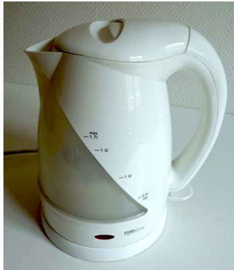
Figure 2.1: The water boiler I use to prepare my morning's coffee and its perceived affordances: the slit on the top cover which fits several fingers, the large handle on the side that invites people to carry it with a single hand rather than grasping the potentially hot main body and the low position of the start button which affords pushing.
