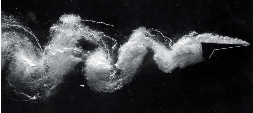
Figure 3.1: Cavitating vortices in the separated wake of a lifting flat plate with a flap; the flow is from the right to the left; Reprinted from [14].
