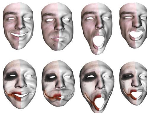
Figure 1: Accurate 3D facial expressions can be animated and transferred in real-time from a tracked actor (top) to a different face (bottom).
