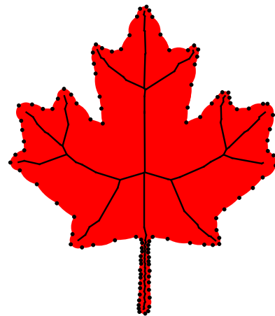
(f) Final result for both our and the standard algorithm: medial axis of the inner Voronoi balls. The standard algorithm needs the steps illustrated on Figure 1(c) and 1(d), our method computes it directly from Figure 1(b)
