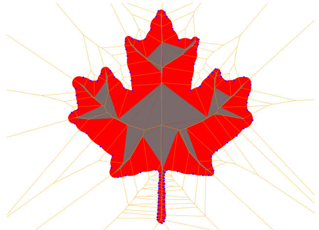
(d) Vertices of the union of balls in blue and their Voronoi diagram in orange
