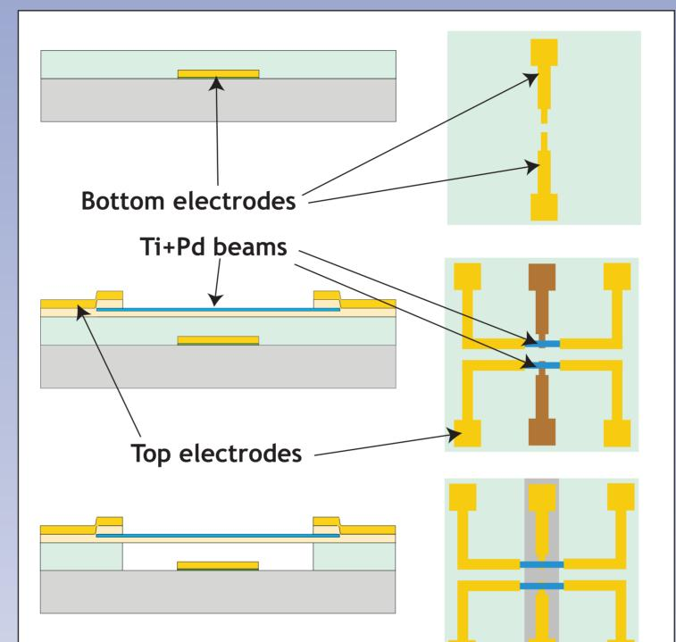
Bottom electrodes (Au) are defined on a pyrex wafer. The wafer is then coated with polyimide or parylene as a sacrificial layer.
