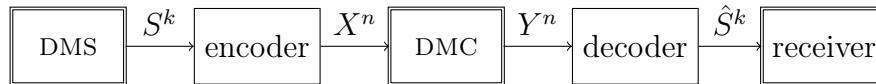
Figure 2.7: A point-to-point communication system consisting of a discrete memoryless source (DMS) with distribution P_S , a discrete memoryless channel (DMC) with transition probabilities P_{Y|X} , an encoder and a decoder.
