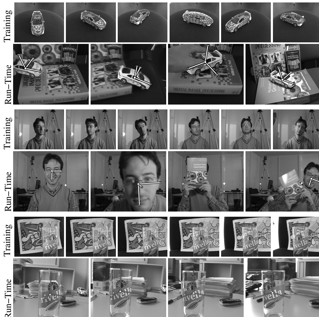
Figure 3.1: Our approach to 3D object detection applied to a toy car, a face, and a glass. In each one of the three cases, we show two rows of pictures. The first represents the training sequence, while the second depicts detection results in individual frames that are not part of the training sequence. We overlay the ellipsoid we use as our initial model on the images of the first row. The only required manual intervention is to position it in the very first image. To visualize the results, we attach a 3D referential to the center of gravity of the ellipsoid and use the estimated 3D pose to project it into the images. Note that, once trained, our system can handle large aspect, scale, and lighting changes. It can deal with the transparent glass as well as with the hand substantially occluding the car. And when a complete occlusion occurs, such as when the book completely hides the face, it simply returns no answer and recovers when the target object becomes visible again.
