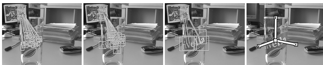
Figure 3.7: Detecting a transparent object with partial texture. The squares in the first three images outline the patches around the features detected at three different scales in a test frame. The straight line segments connect the feature with the corresponding one in a frame of the training sequence. Since during training the system learned which parts of the patches are meaningful as shown in Figure 3.3, the image features can be recognized even if the patch overlaps the background or the transparent parts. As shown in the fourth frame, the glass is successfully detected.
