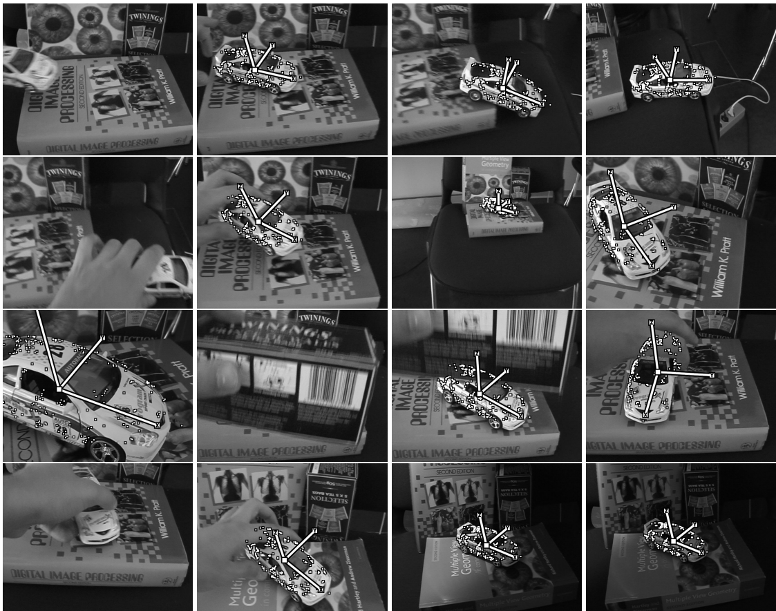
Figure 3.5: Detecting the car in a sequence that involves abrupt motions, large scale and lighting changes, and very substantial occlusions. To visualize the results, we attach a 3D referential to the center of gravity of the initial ellipsoid and use the estimated 3D pose to project it into the images. We also overlay the projections of the harvested object feature points. The toy car is successfully detected in all frames except those where it is almost entirely occluded. And, because the object is re-detected in every frame, the system easily recovers after such a failure.
