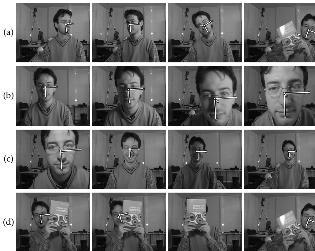
Figure 3.6: Face results. Note that by contrast with previous face detection approaches, the face pose can be retrieved under (a) large rotations, (b) scale and lighting changes, and (c) different facial expressions. (d) After the occlusion by the book, the algorithm automatically recovers.
