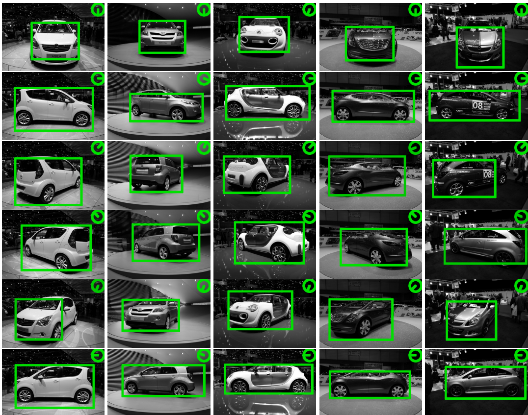
Figure 4.1: Sample detections from the test set. The green rectangle depicts the recovered bounding box and the estimated viewpoint is indicated inside the green circle at the top-right corner. A front facing car is indicated by a downward pointing line. Despite the challenging lighting conditions and changing backgrounds our approach can correctly localize cars and estimate their pose.
