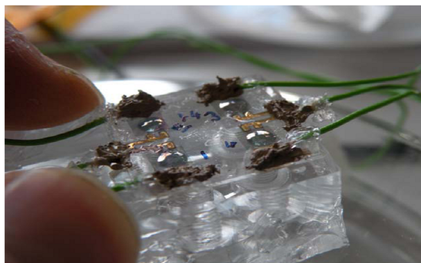
Figure 10. A completed device with a set of four membranes, which can be used as three lenses and one actuator, or one lens and three actuators. For scale, two fingertips are visible on the left.
