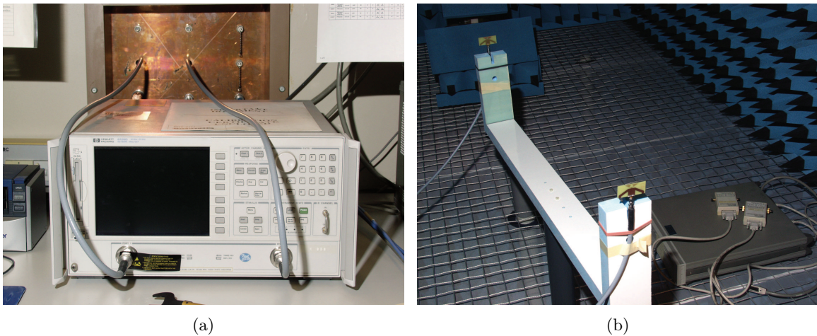
Figure 4.9.: Measurement setup: (a) Setup of HP 8720D Network Analyzer outside anechoic chamber, (b) Antennas in foam support and calibration kit inside anechoic chamber.
