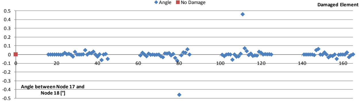
Figure 13. Angle between the midspan nodes after individual cable damage and no damage
