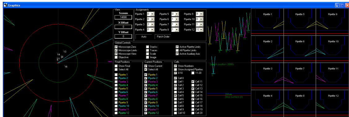
Figure 2-3 Graphic representation of the positions of 12 electrodes in multiple views and top-view representation of positions of cells of interest (left panel).
