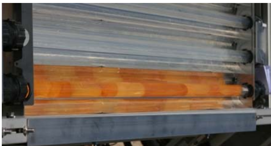
Figure 6.4 Picture of PVF f -TiO 2 -Fe oxide films in the CPC photo-reactor
