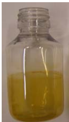
Figure 4.15 Photography of PET b f -TiO 2 -Fe oxide used in this study
