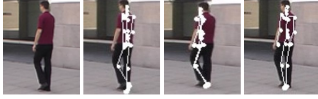
Figure 4.11: Appearance based refinement process. The images are from left to right the input image, the initialization given by the interpolation process, the result obtained without using a background image, and finally the result obtained as proposed. Whole parts of the body can be missed when the background is not exploited.
