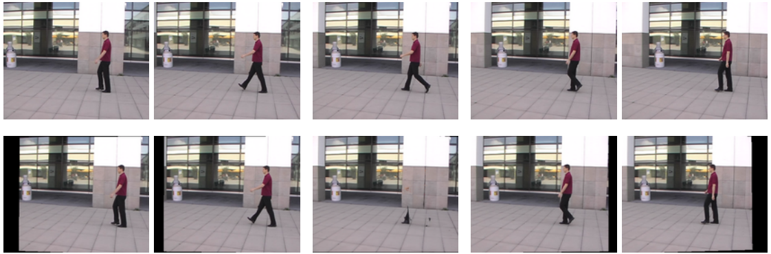
Figure 4.10: Synthesizing a background image. First row: The central image is the reference image whose background we want to synthesize. The other four are those before and after it in the sequence. Second row: The same four images warped to match the reference image. Computing the median image of these and the reference image yields the central image, which is the desired background image.
