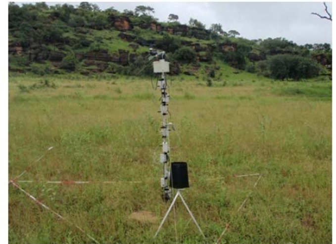
Fig 2. Wireless sensing Device, Sensorscope used for observation in agricultural field.
