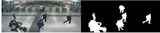
Figure 5. An example of simulated image, with its corresponding foreground ground truth mask.
