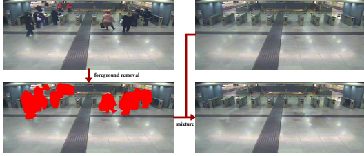
Figure 4. Generation of a Background and Shadow frame (BSF) (bottom right), by filling the holes in the bottom left image with the content of a background image (top right).
