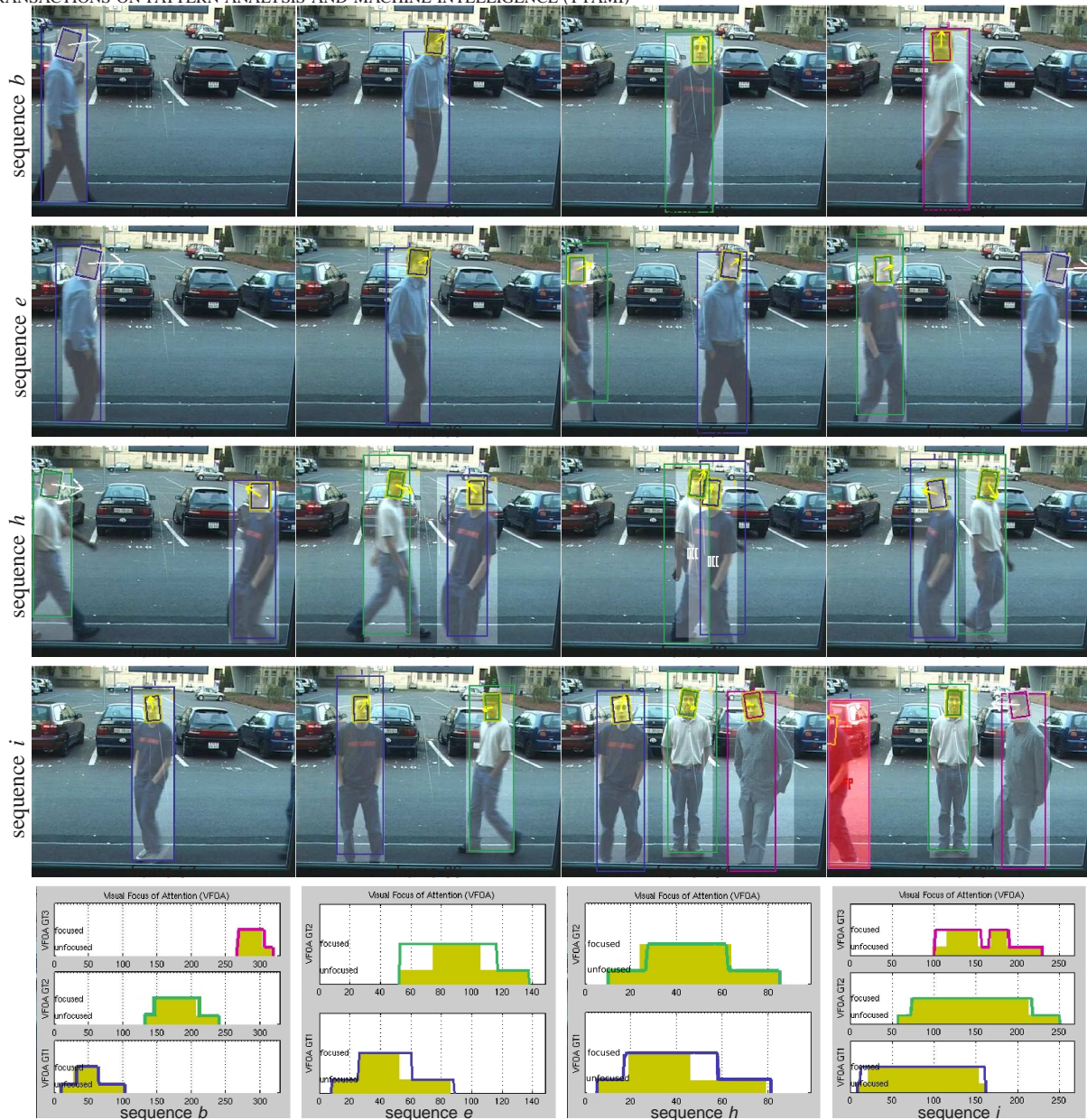
Fig. 9. Tracking and VFOA-W results for sequences b , e , h , and i . Tracking results appear as boxes around the body and head. A yellow pointing vector/head border indicates a focused state, a white pointing vector/head border indicates an unfocused state. The ground truth appears as shaded boxes for the head and the body (the head area is shaded yellow when labeled as focused and gray when labeled as unfocused ). VFOA-W results for the GMM model appear at the bottom. The yellow bars represent the ground truth (raised indicates a focused state, lowered indicates unfocused , and no yellow bar indicates the person is not present in the scene). GMM VFOA-W estimates appear as colored lines. VFOA-W performance was nearly perfect for b , with good event-based recognition in all sequences. Mild frame-based VFOA-W recognition errors occurred in e , h , and i . Frame 162 of sequence i shows a FP error generated as a tracker was placed where no ground truth was present.
