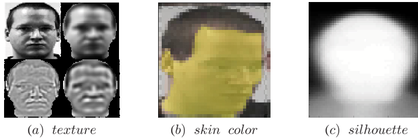
FIG. 5 – (a) Texture is used to estimate the head-pose by applying three filters to the original image (upper left). These filters include a coarse scale Gaussian filter (upper right), a fine scale Gabor filter (lower left), and a coarse scale Gabor filter (lower right). (b) Skin color models help to keep the head-pose robust in presence of background clutter. (c) A silhouette model is responsible for localizing the head’s spatial component.
