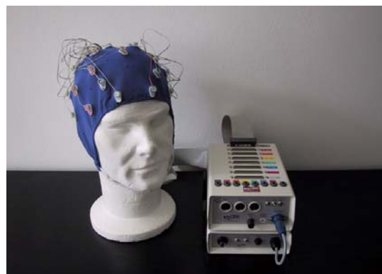
Figure 2. Portable EEG system used at the IDIAP Research Institute. It is a commercial BioSemi ActiveTwo system
