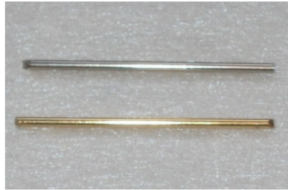
Figure 1.2: An 18-carat white gold alloy containing 12.5 weight-% palladium (Au 5125, top) and an 18-carat yellow gold containing 12.5% silver (Au 318, bottom).
