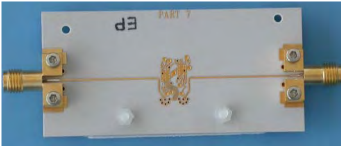
Fig. 8 Picture of the complete ERC measured
