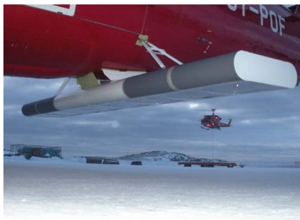
Fig. 1 Array installation on the belly of a Twin Otter aircraft.
