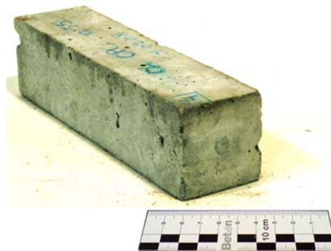
Fig. V-9. Visual appearance of P-0.55 after 386 days of exposure under pH-control.
