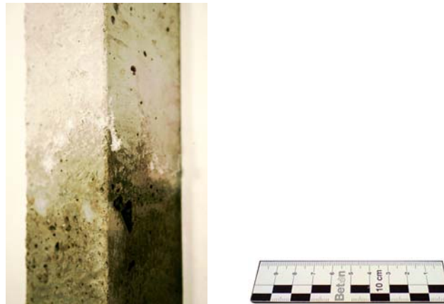
Fig. V-19. Typical visual appearance of the laboratory micro-concretes after 175 days of exposure in semi-immersion.
