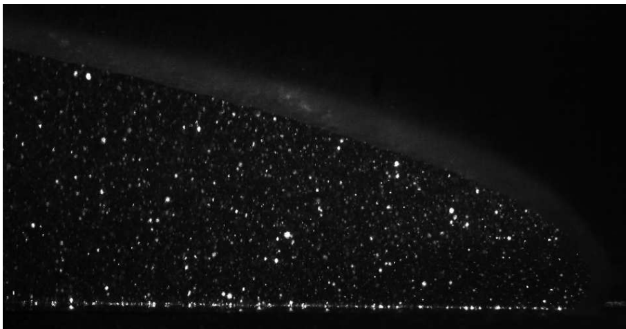
Figure 6.1: Flow front (dam-break experiment) of a concentrated and refractive-index-matched suspension with a particle volume fraction of 0.55 and an inclination of 0^\circ , images have been taken from the side at a depth of 20 mm into the fluid. The suspension flows from left to right and the bright dots are marked particles advected by the fluid, which are used as tracers to infer fluid velocity.
