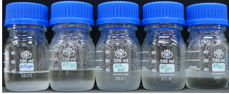
Figure 4.8: The one week sedimentation experiment: from left to right, fluid densities of 1.1830; 1.1835; 1.1840; 1.1850 and 1.1865 g/cc. The bright part is due to a concentration of particles while the dark part means that the corresponding local volume is almost free of particles. In the 1.1840-g/cc sample, no demixing could be noted (in this experiment, particle and fluid were only density matched to allow a better sedimentation visualisation)
