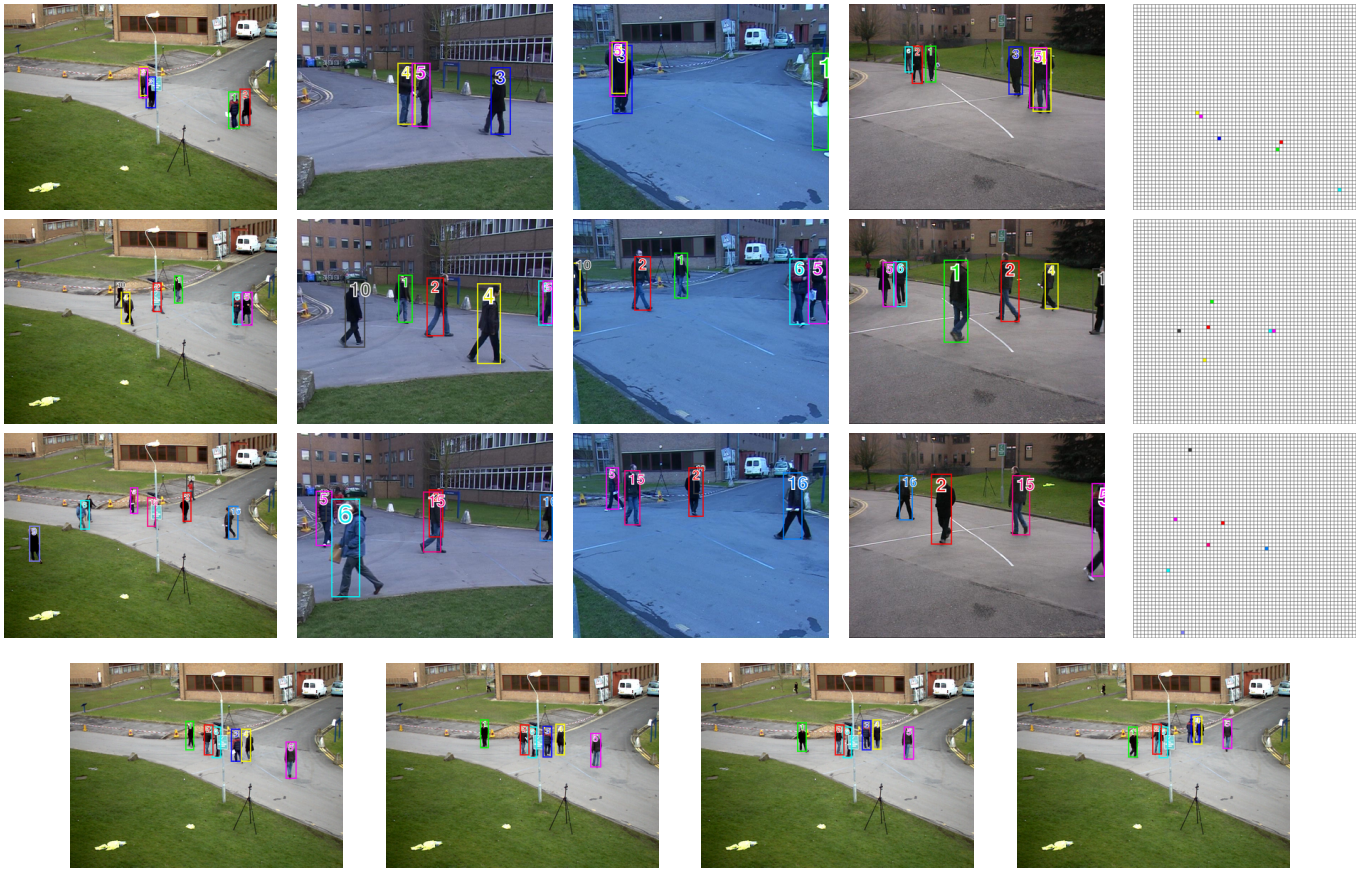
Figure 7: Some results of our LP-based tracker on a PETS 2009 sequence. Each of the three first rows shows a different time frame of the sequence. The first four columns display multi-camera tracking results in four of the five available camera views. The right-most column represents the corresponding detections on the ground plane. The last row shows four result frames in the monocular context. Since the people identities are color coded, this figure is best viewed in color.
