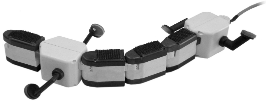
Fig. 5: The prototype of salamander robot built with the first generation elements
