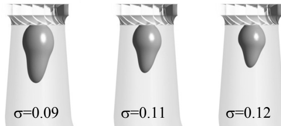
Fig.5 Variation of the vortex rope volume as function of the Thoma number
